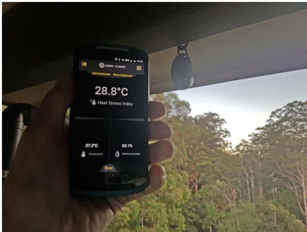
Kestrel Drop D2, and smartphone with Kestrel LiNK app, showing (at top) heat index, (and below) temperature and relative humidity
